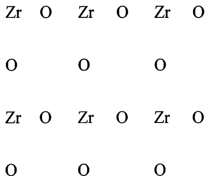
FIG. 4. Surface of cubic ZrO_2 . Zr, zirconium site; O, oxygen site.
